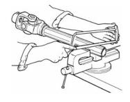
ASSEMBLE THE SHIELDS ON EACH HALF, THEN CUT THE TUBES THE SAME LENGTH AS THE SLIP TUBES.
